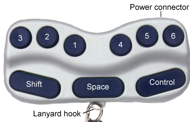
Illustration 1: Picture of the BraillePen Slim with all features labelled
